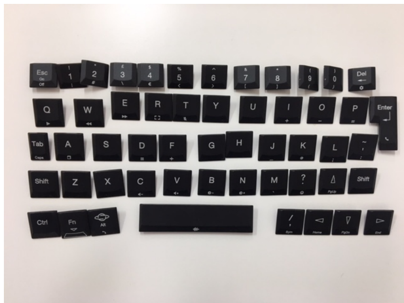
Photo 6: Photo of all removed keycaps laid out as they were on the original keyboard to aid reassembly.
