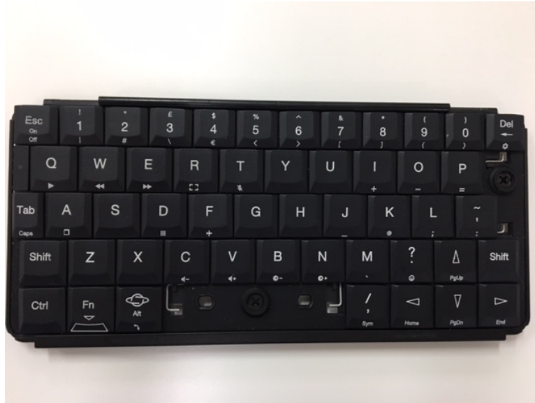
Photo 10: Photo showing the keys all back reassembled onto the keyboard with only the SPACEBAR and ENTER keys left to reapply..
