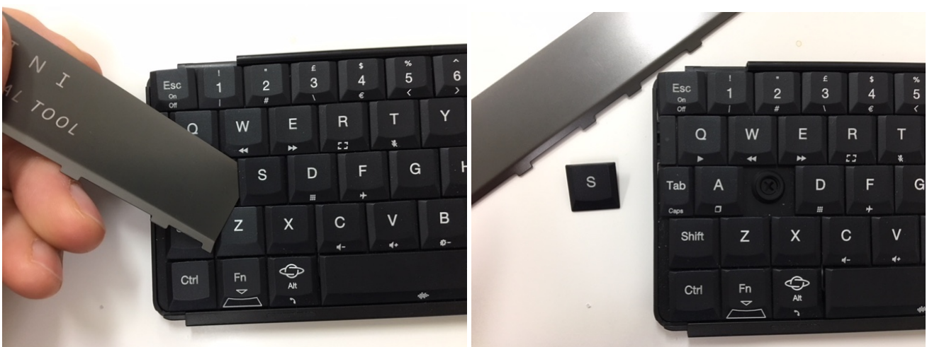
Photo 2 & 3: Photo of an example flat tool (eg Cover Removal Tool) under one of the keycaps and then the removal of the S key.
