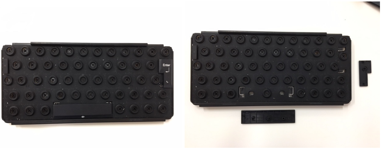
Photo 4 & 5: Photo showing the keyboard following removal of all keys apart from SPACEBAR and ENTER and the difference between the normal keys and SPACEBAR and ENTER keys.
